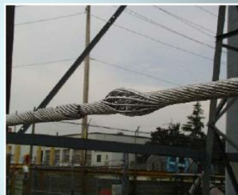
Figure 23: Birdcage in ACCR at 1200 kA 2 s (300-340°C)
