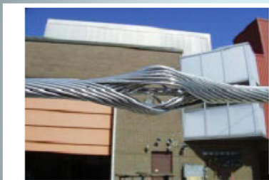
Figure 23: Birdcage in ACCR at 1200 kA 2 s (300-340°C)
